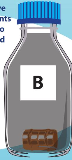
Heating oil will darken and degrade over time when in contact with the copper lines in heating oil systems.
