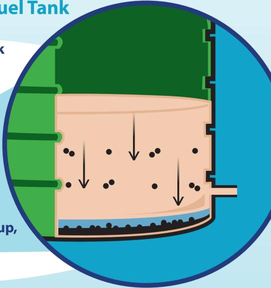
Over the years, the sludge will build up. Upon re-filling a near empty tank, the sludge may be stirred up, blocking the line filters.
